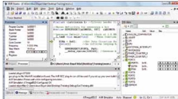
Fig. 4: AVR Studio window for simulation
