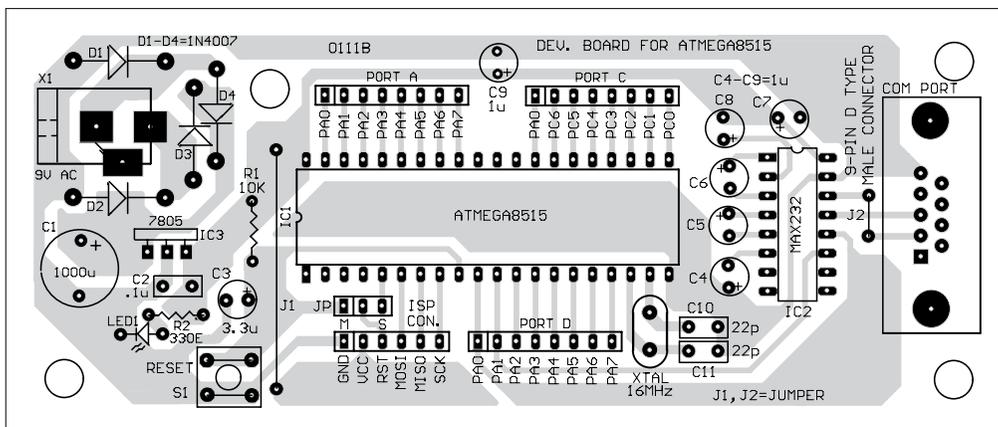
Fig. 8: Component layout for the PCB
