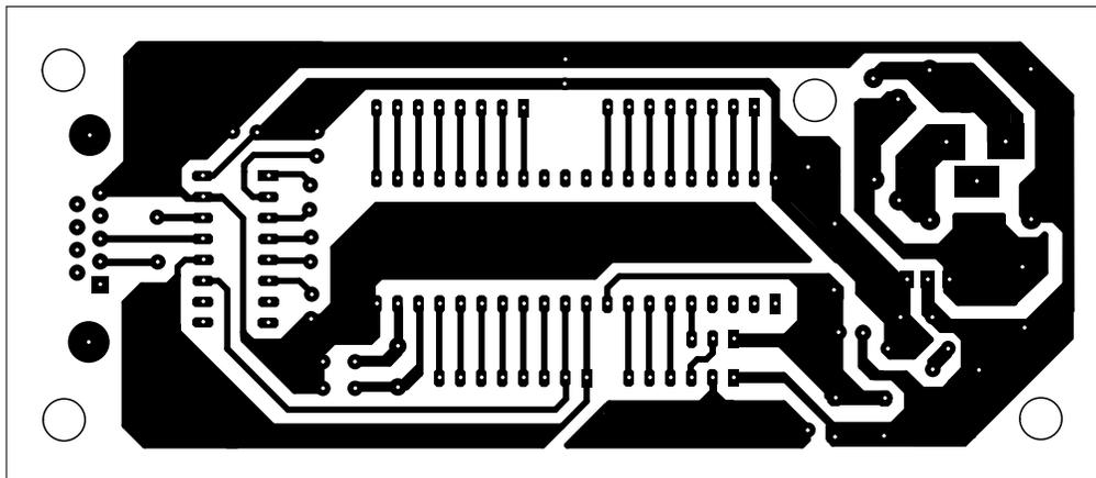
Fig. 7: An actual-size, single-side PCB for the ATmega8515 development board
