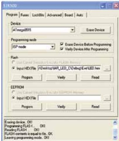
Fig. 6: STK500 window for data downloading into microcontroller
