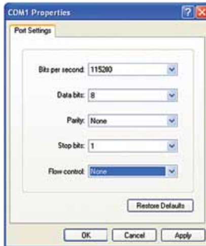
Fig. 9: HyperTerminal windows for selection of baud rate, data bits, parity, stop bits flow control
