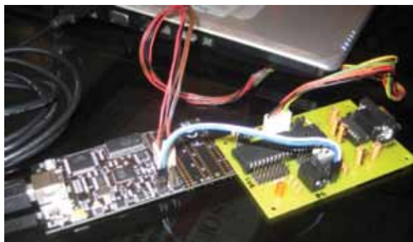
Fig. 5: Burning the hex code into the programmer board microcontroller
