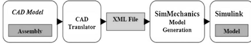
Fig. 3 Translating CAD model to SimMechanics
