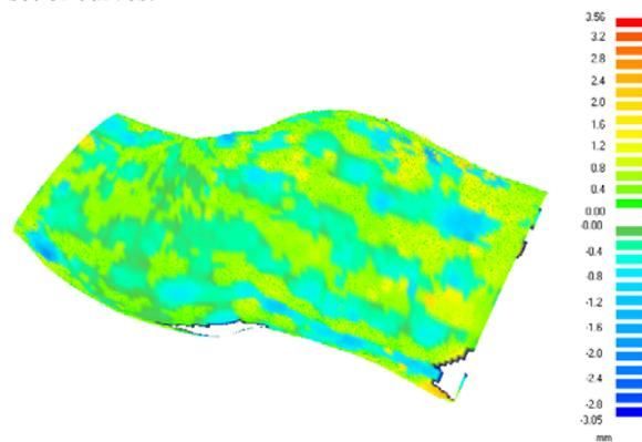
Fig 10: Surface to cloud difference analysis.
