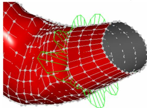
Fig 11: Continuity check at the joining of two surfaces.
