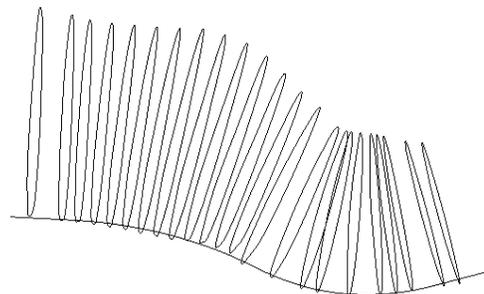
Fig 5: Set of closed B-Spline curves fitted over sectioned cloud points.
