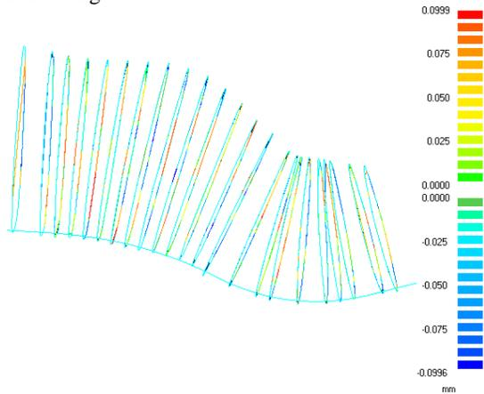
Fig 6: Curve to cloud difference analysis
