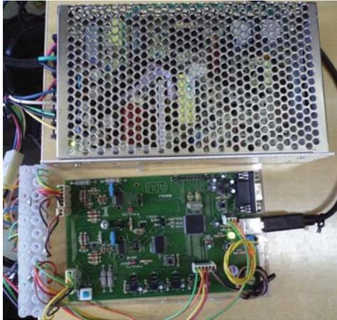
Figure 4. Assembled PCB with power supply
